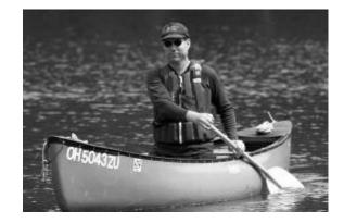
**A.** Whitewater Canoe: A canoe designed for whitewater will have more rocker and more flotation than its flatwater counterpart.
