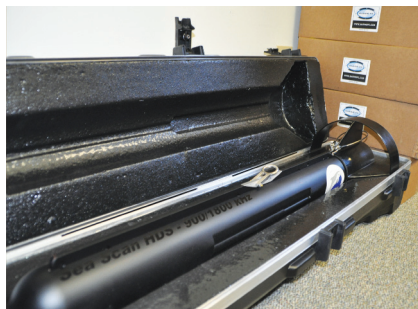
This torpedo-shaped sonar is towed behind boats and can reach depths of 2,000 feet to give agents a visual of the water bottom when looking for evidence, sunken vessels or deceased bodies.
