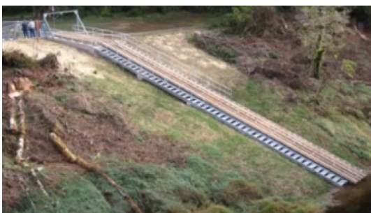
This specialized boat access provides a "skid" to assist movement of nonmotorized boats up and down a steep embankment.
